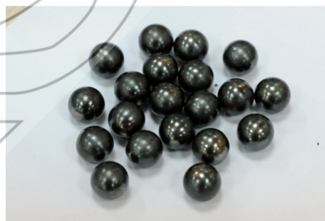
图7 断油试验故障轴承钢球 Fig.7 Failure bearing balls of oil-off test
